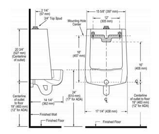
NOTE: ADA urinal rim height requirements allow all heights 17<sup>e</sup> and below. Sloan strongly recommends roughing in the drain to achieve a 16%<sup>e</sup> rim height or less to ensure compliance.
